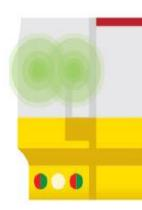
The high Brightness LED flashes once and the device beeps once. Hold the magnet next to the test area for three seconds. A second beep indicates that the device is in full function test mode. The battery LED and the GPS LED flashes every three seconds to indicate the battery and GPS locating status: • A green battery LED indicates that the battery has passed the test. A red battery LED flashing indicates that the battery has low
