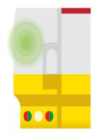
The high brightness LED flashes and the device beeps once indicating that the device is in battery life test mode. A green flash indicates that the battery has passed the test. A red flash indicates that the battery has low power and needs to be replaced. The device flashes three times and beeps once to end the test.
