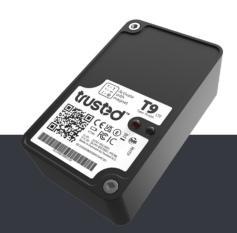
This **RHTP** edition features high precision humidity, temperature and air pressure monitoring in one device.
